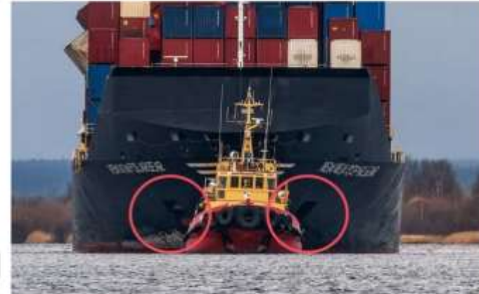
The Newnew Polar Bear in Arkhangeisk, seen missing its portside anchor. Source: Vitaly V/ fleetphoto.ru/Yle
